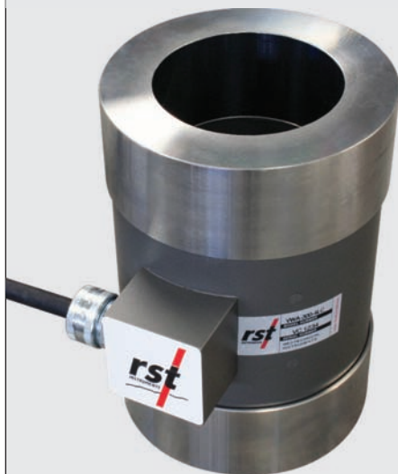
Annular load cell shown with top and bottom platens.
